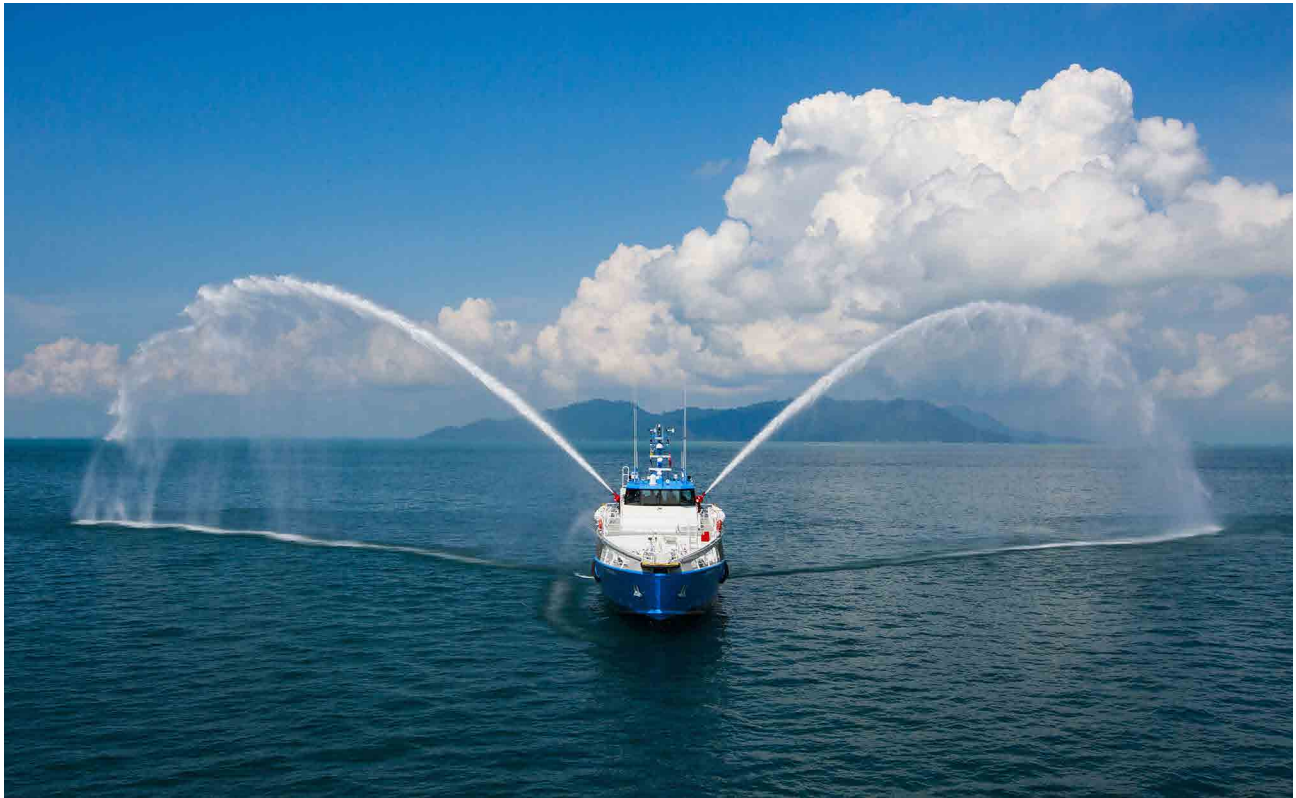
Rapido Gee testing fire pumps (Photo courtesy Incat Crowther)
