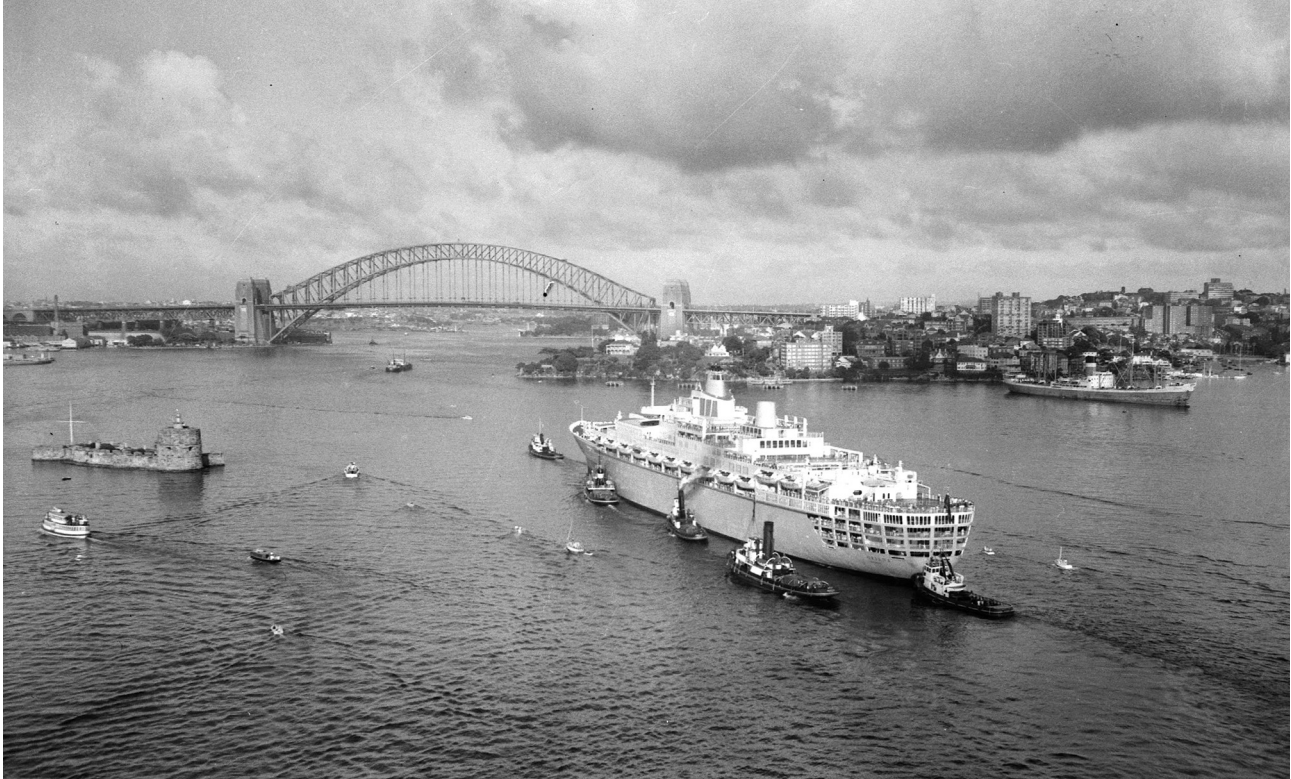
The last of the Orient Steam Navigation Company's liners, Oriana , arriving in Sydney for the first time on 30 December 1960. With a displacement of 39 100 t she was the largest liner ever built in England and could carry 688 first-class and 1496 tourist-class passengers with a crew of 899. She was designed and built by Vickers at Barrow-in-Furness (Photo Australian National Maritime Museum, Gervais Purcell collection)
