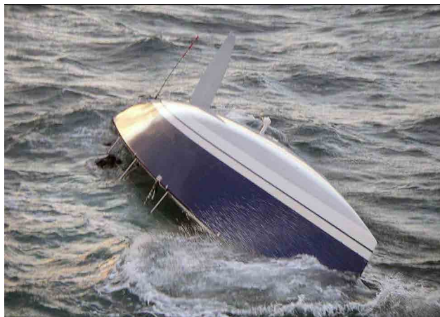
Hooligan V after loss of keel (Photo from Marine Accident Investigation Branch Report 19/2007)
