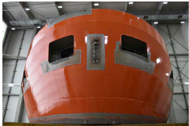
The stern module of RSV Nuyina (Photo by Michiel Jordaan, courtesy Australian Antarctic Division)
