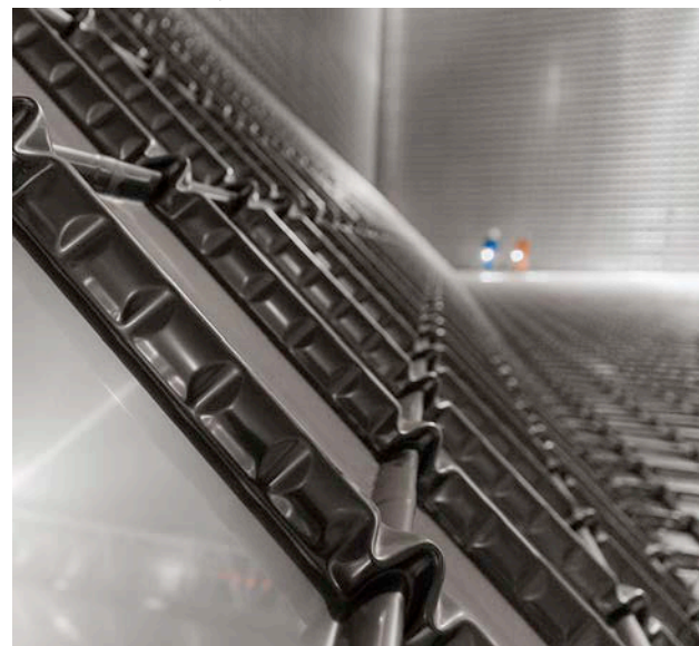
Workers inspecting the tank of an LNG carrier equipped with GTT Mark technology (Photo courtesy BV)
