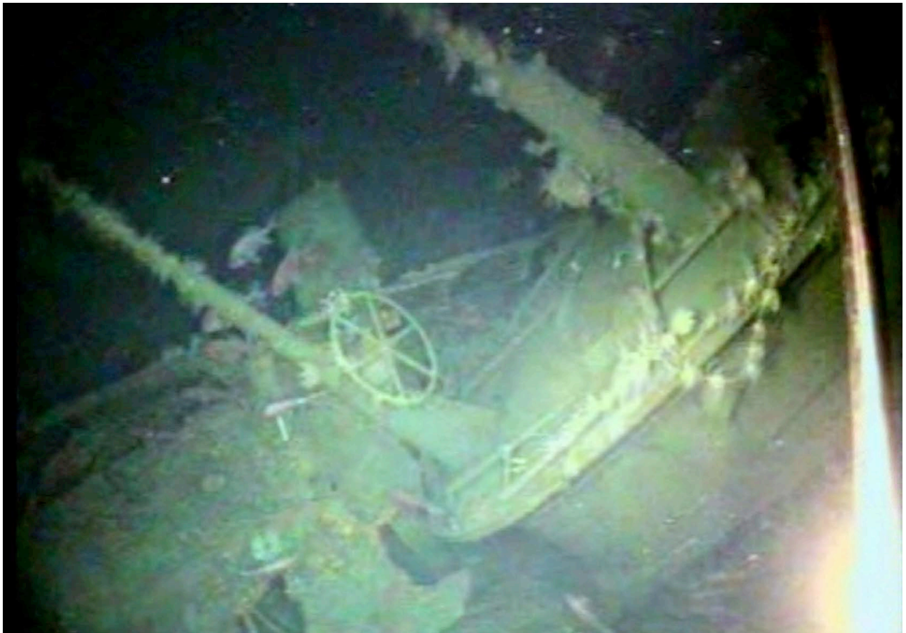
The conning tower of HMAS AE1 showing the two periscope standards and the submarine's surface helm (Photograph Fugro Survey, courtesy Department of Defence)
