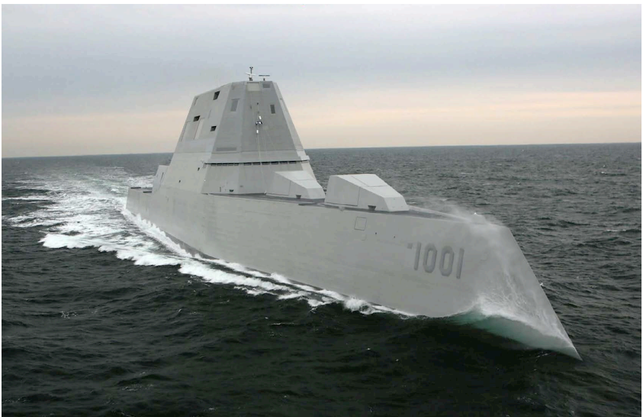
The second of three Zumwalt-class destroyers for the US Navy, the future USS Michael Monsoor , completed acceptance trials on 1 February. The construction of the 14 829 t, 182.9 m long ship began at Bath Iron Works in Maine in March 2010 (US Navy photograph)
