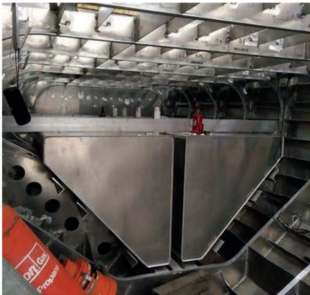
Forward fuel tanks installed on Excalibur (Photo from Team Britannia Facebook website)
