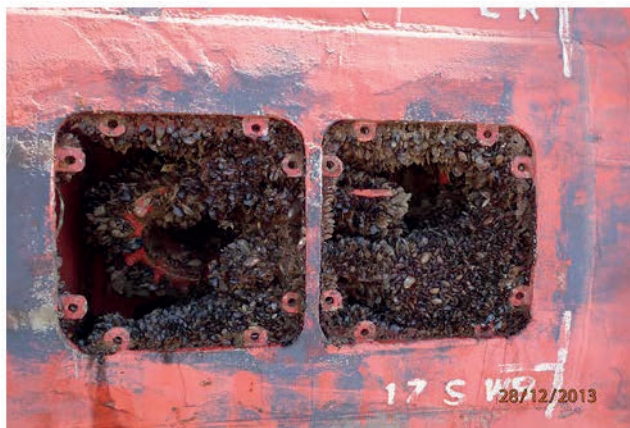
Fouling in a sea inlet on an OSV in Bass Strait (Photo courtesy John Lewis)
