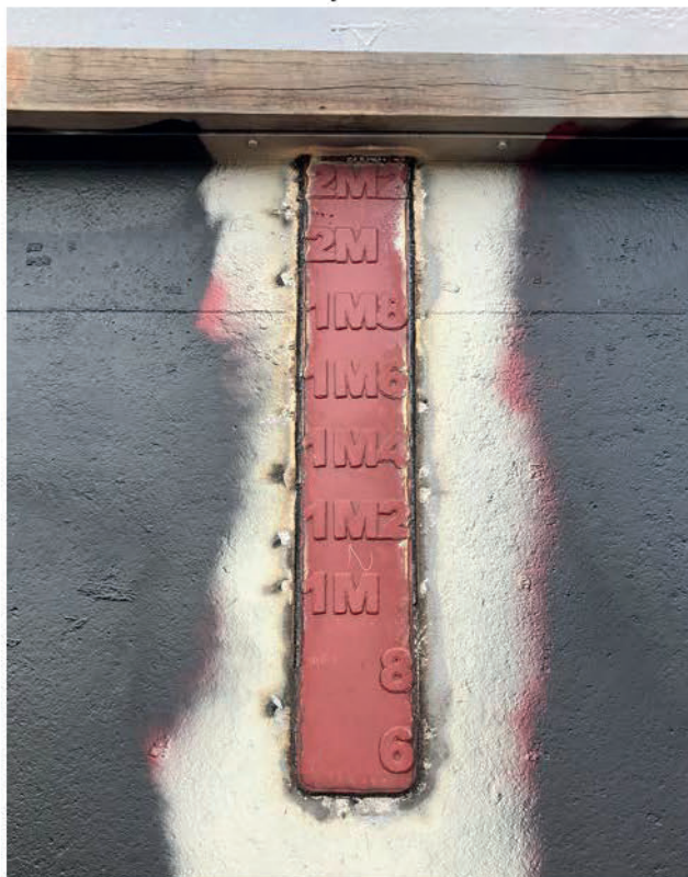
New metric draft marks (Photo courtesy Noakes Group)
