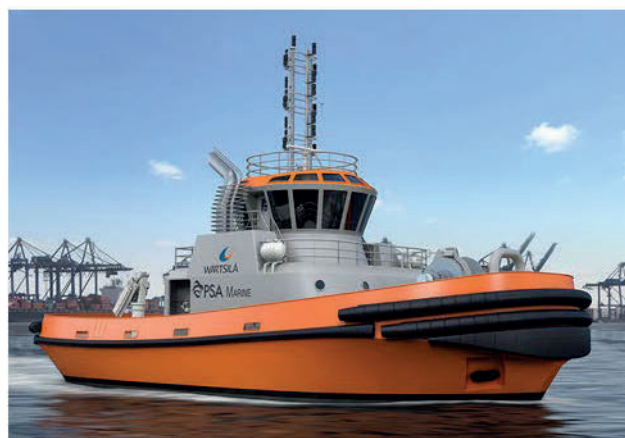
The Wärtsilä designed and equipped LNG fuelled harbour tug (Image courtesy Wärtsilä)
