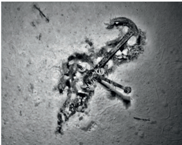
An Admiralty type anchor with iron stock at the IOS-001 wreck site (Image Fugro/ATSB)
