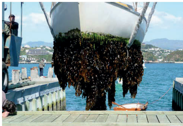
Fouling on a yacht left too long in the water! (Photo courtesy Biosecurity NZ)
