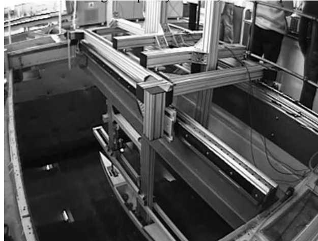
Mechanism for imposing unsteady motion onto the mean carriage speed (Photo courtesy Sandy Day)
