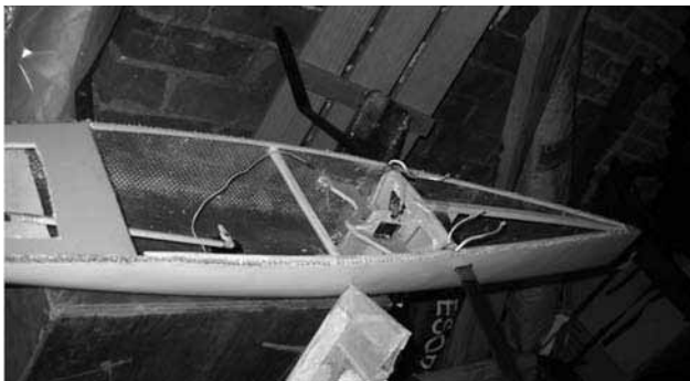
Figure 9 — Hull No. 4 showing Nomex honeycomb core foils later moved to lower position
