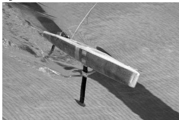
Figure 12 — Model foilborne with tips just breaking the surface at 1.74 m/s
