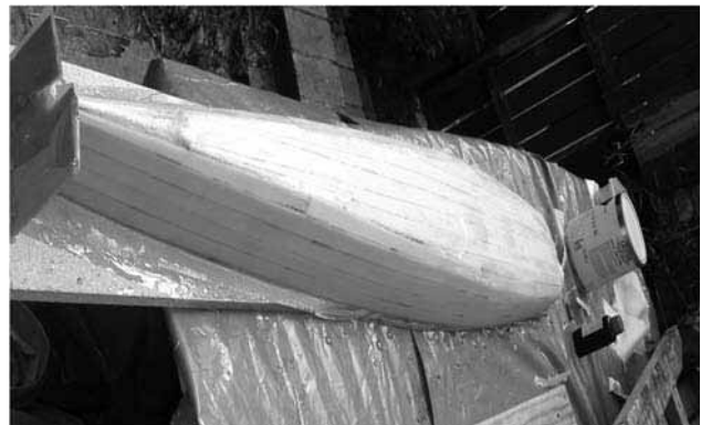
Figure 6 — Plug under construction, still attached to building frame
