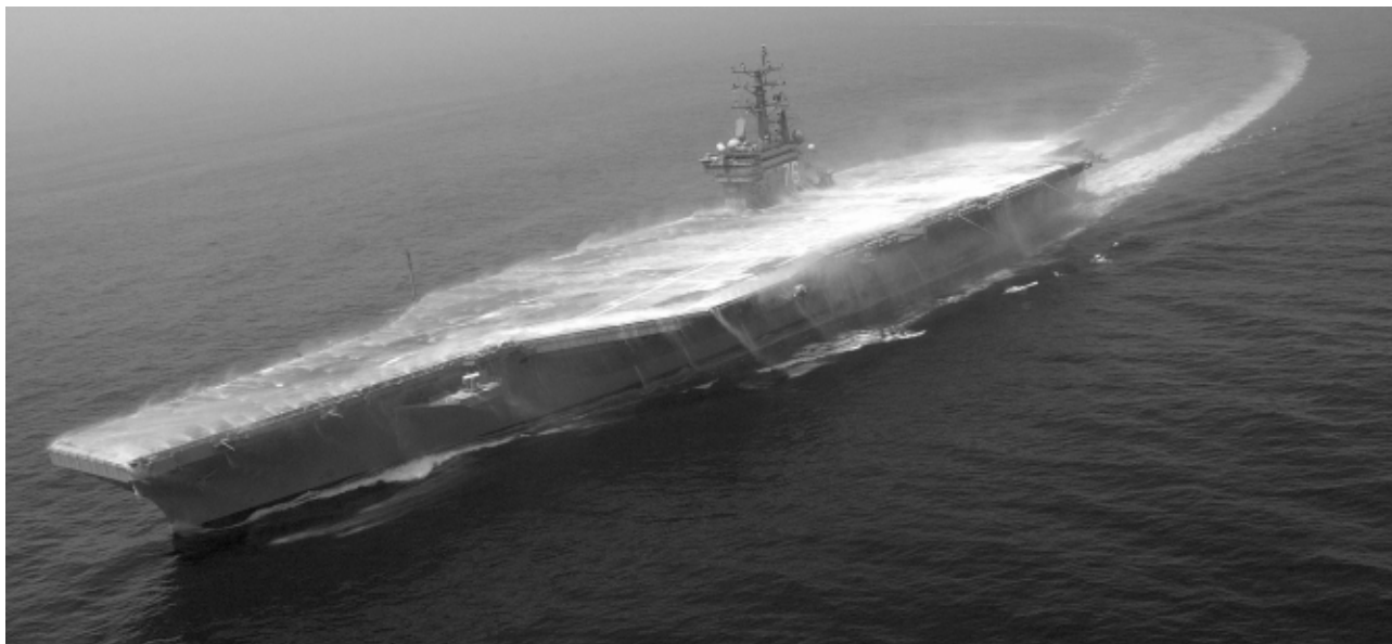
The US Navy's newest Nimitz-class aircraft carrier Ronald Reagan tests its counter-measure wash-down systems (CMWDS) during builder's sea trials off the coast of Virginia. CMWDS includes a series of sprinklers in vital areas throughout the ship to help contain the spread of fire or chemical, biological or radiological attacks.
