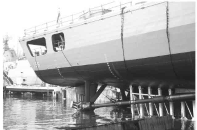
HMAS Toowoomba showing the zero-thrust propellers used for trialing the engines, (Photo Phil Helmore)
