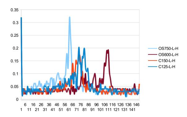
This still proved difficult to see defining differences, as different models, due to different hull shapes, show multiple peaks at different parts of their transition. It is noticeable however that the OS750 has the overall highest amplitude, the C125 and OS600 similar peaks, and the C150 the lowest peak
