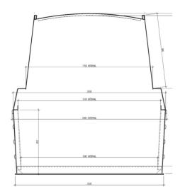
I note that concentration within these parameters has been on cost reduction with limited plate bending at bow and stern. The latest designs have design draughts at 20" (0.5m) or less leading to instability in tidal waters.
