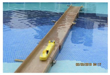
The test rig pictured above shows a trough 9.6m long, 0.6m width built out of ply set at the bottom of a partly filled swimming pool. The model is heading away from the viewpoint of the photographer. The two timing gates are clearly visible.
