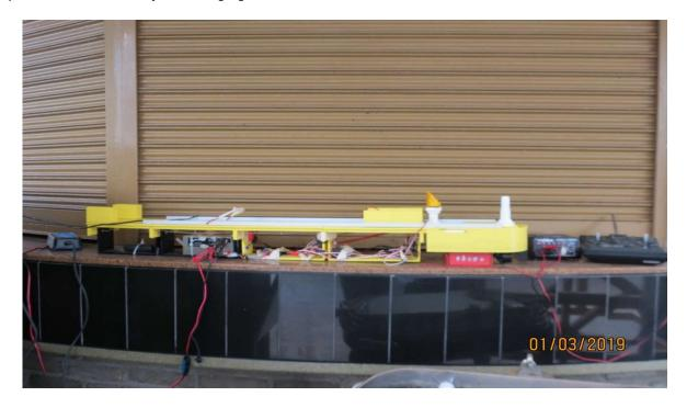
Propulsion deck shows battery in the bow, radio receiver in the centre and a stern section with Schottel drive below propped on a box to reduce flex. The entire deck with battery/drive/radio controls was designed to lift off and be placed on any of the four models.
