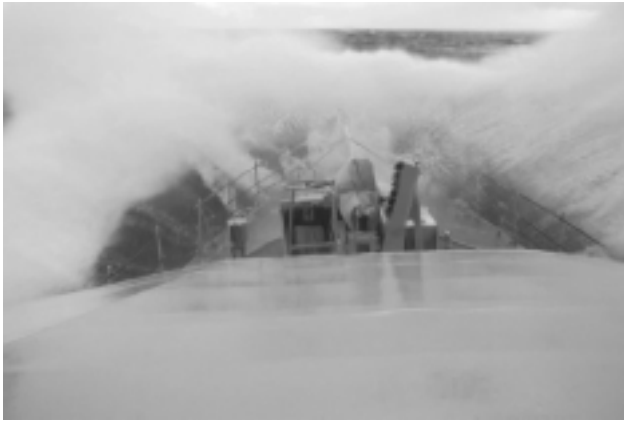
HMAS Warrnambool demonstrating the advantages of bow flare (RAN photograph)
