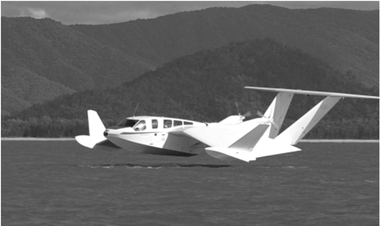
The Eight-Passenger FlightShip 8 flaring at 80 knots near Cairns, Queensland (Photo courtesy David Philp of FlightShip Ground Effect)
