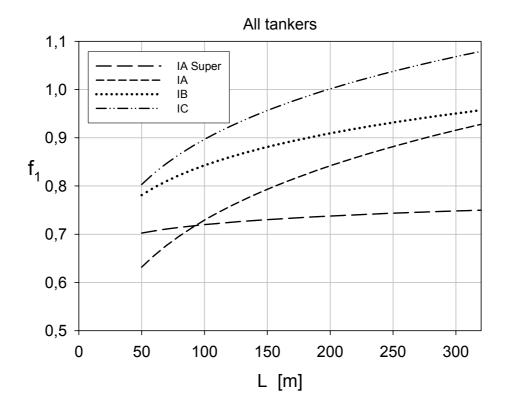
This plot suggests that some changes are required. The form of the upper limit of  $f_I$  should not be larger than one (=1.0) – thus the curve for ice class IC should be corrected. Also the curves for ice classes IA and IA Super cross at ship length of about 100 m – this is also not correct.
