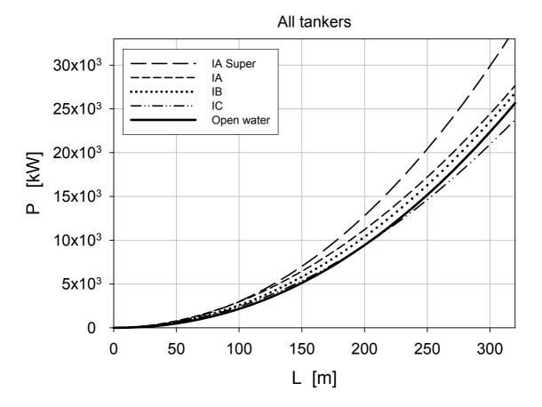
The final form of the correction coefficient  $f_I$  is presented in the table below (unit for the power is kW). The form of the coefficient is the average open water power calculated using the ship's actual length divided by the actual installed ship power, i.e.
