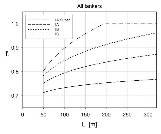
The final form of the correction coefficient  $f_1$  for tankers can now be presented. This uses both the above definitions. Thus the power correction coefficient is given for each ice class separately as (units kW and m):
