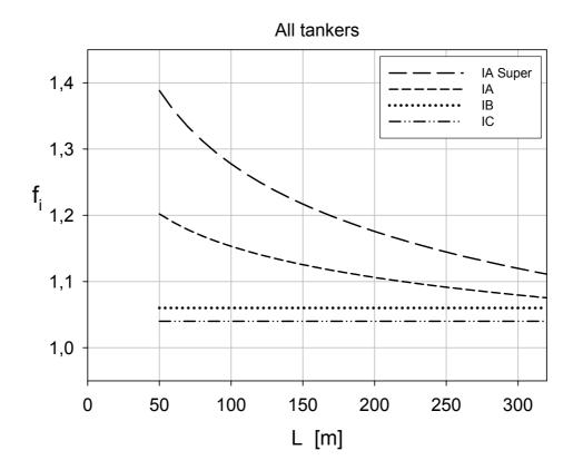
The final form of the correction coefficient  $f_i$  can now be presented. This uses both the above definitions. Thus the capacity correction coefficient is given for each ice class separately as (units dwt and m):
