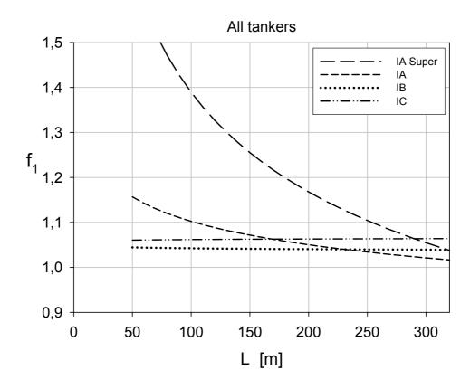
As these curves are calculated from direct regression curves, several errors can be pointed out. For tankers the curves for ice classes IB and IC are in inverse order to that expected and also the trend with length is too pronounced for higher ice classes.
