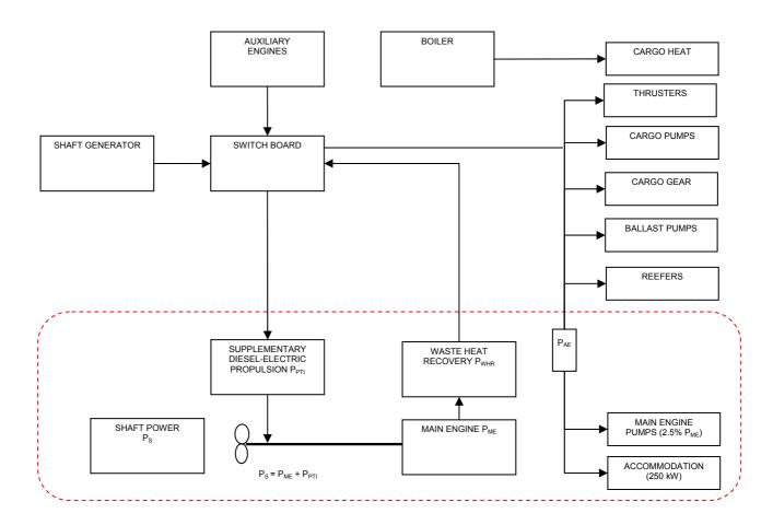
The power contributions in the dotted box should be considered by the new ship design CO<sub>2</sub> index, and the power contributions outside the dotted box should be excluded. Auxiliary power is generated by the auxiliary engines and may be supplemented via the switchboard by additional power from a shaft generator or from waste heat recovery systems.
