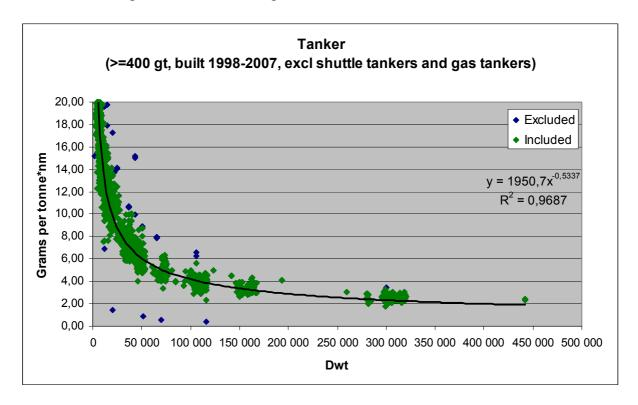
Shuttle tankers are tankers which carry crude oil from offshore fields to onshore storages. They are quite different from ordinary tankers with much higher installed power. They do not cover long distances, are equipped with dynamic positioning systems and are designed for complex operations in rough seas and are therefore excluded.
