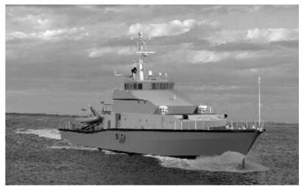
The proposed Inshore Patrol Vessel is 340 tonnes displacement, 55m long x 9m beam and capable of up to 25 knots, with a maximum range of 3000 nm. The ships will have accommodation for a core complement of 20 personnel plus provision for four government agency officers and 12 additional personnel.
