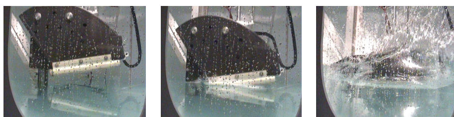
Figure 4. Typical slamming event in SSTS
