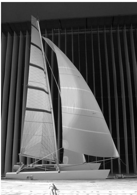
The Test Rig Catamaran at the Auckland University Twisted Flow Wind Tunnel
