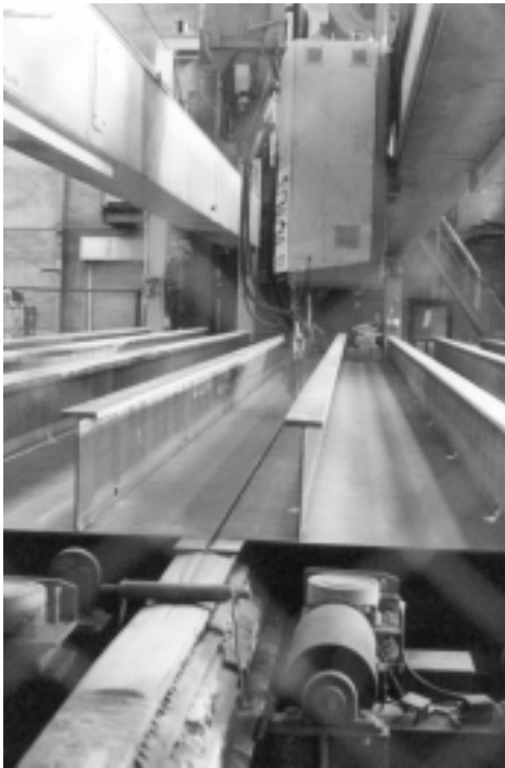
Figure 2. One of the automatic welding machines in operation (Photo courtesy Ian Raymond)
