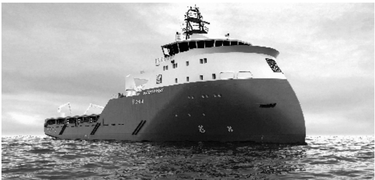
This new anchor-handling tug supply vessel of Ulstein AX104 design will be equipped with generating sets, tunnel thruster, steerable thrusters, control system and seals from Wärtsilä Corporation (Image courtesy Wärtsilä)
