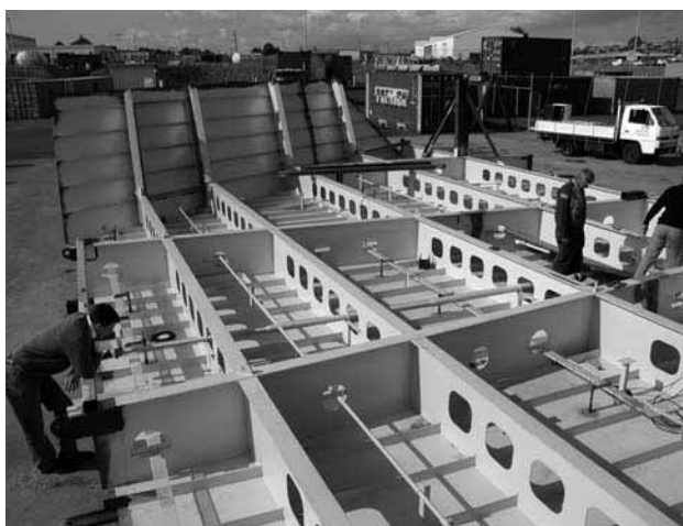
New structure for the Spirit of Tasmania modifications under construction (above) and ready for erection (below) (Photos courtesy Lightning Naval Architecture)
