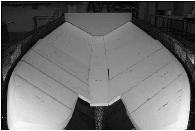
Figure 2 Kitted hull core placed on outer skin in mould
