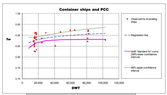
Draft "standard  $f_W$ " curve for container ships and PCC  $f_W = 0.01256 \ln(DWT) + 0.7413$
