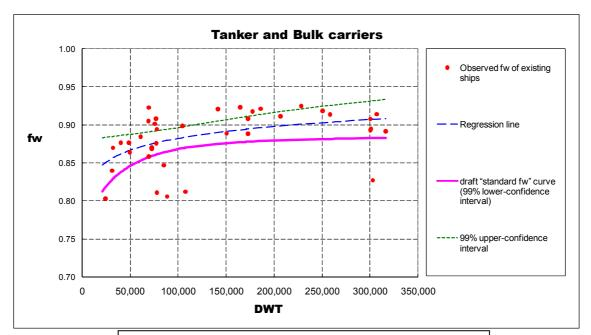
Draft "standard  $f_W$ " curve for tanker and bulk carriers  $f_W = 0.02423 \ln(\text{DWT}) + 0.5830$
