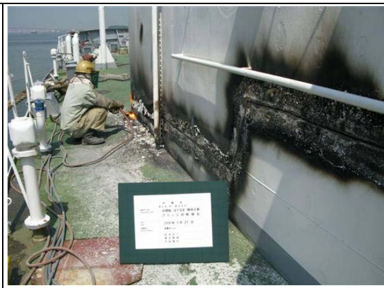
Cutting accommodation structure along the pre-cleaned part of plates
