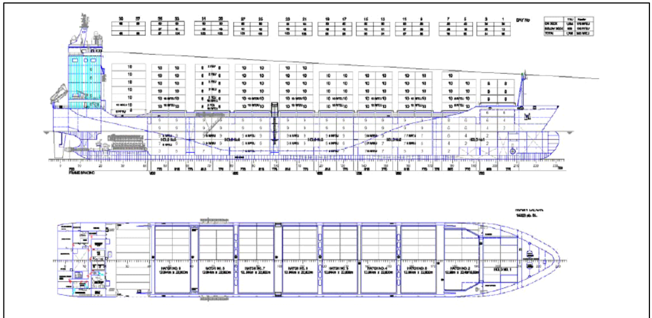
Figure 1: Feeder vessel – General arrangement plan, side and top view
