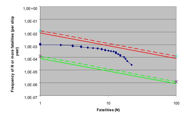
FN diagram for IACS class general cargo ship. Boundaries for intolerable and negligible risk calculated on basis of MSC 72/16 using updated figures for economic value and two q-values (dashed line: 1 and continuous line: 0.68).
