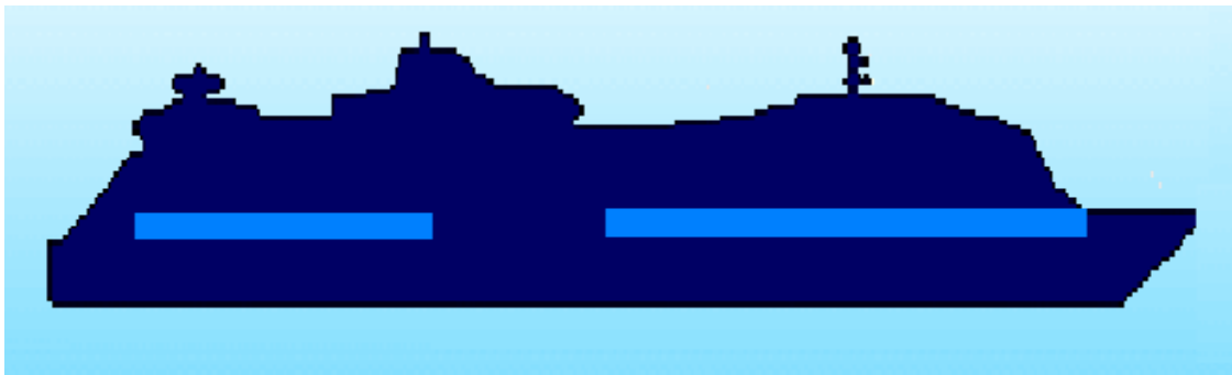
Figure 3 Approximate position of added buoyancy compartments. For illustration purposes only.
