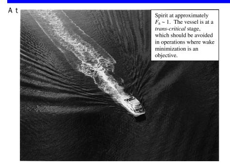
Figure. 3. Photograph of Spirit slowing down and passing through the transcritical speed. Note the large, long waves building alongside the vessel.
