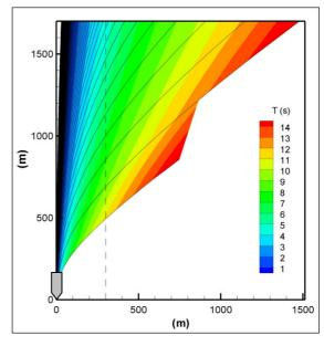
Figure. 1b. Wake period for 38 knot vessel in finite depth water
