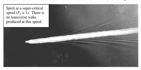
Figure. 4. Photograph of Spirit at a super-critical speed. Note only diverging wakes are present.
