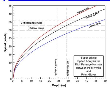
Figure. 5. Critical speeds analysis for Rich Passage Narrows.
