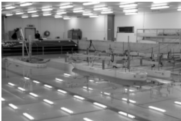
Figure 1 — Ship models set up for the Parker Point configuration (Photo courtesy AMC)
