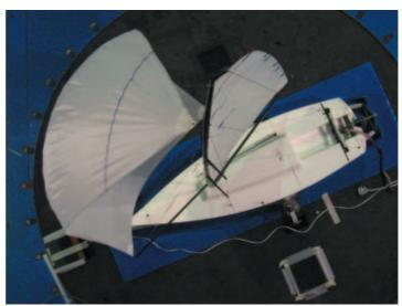
Symmetrical fractional spinnaker tested in the TFWT
