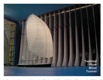
Volvo Ocean 60 model in the Twisted Flow Wind Tunnel of The University of Auckland with flow twisting vanes upstream of the model
