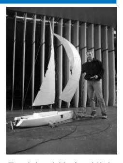
The typical mast height of a model in the TFWT is about 2.3 metres
