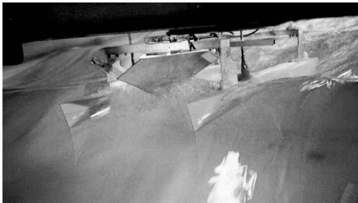
A typical semi captive model test. In this instance the model is being tested with a Vee shaped cross deck bow structure
