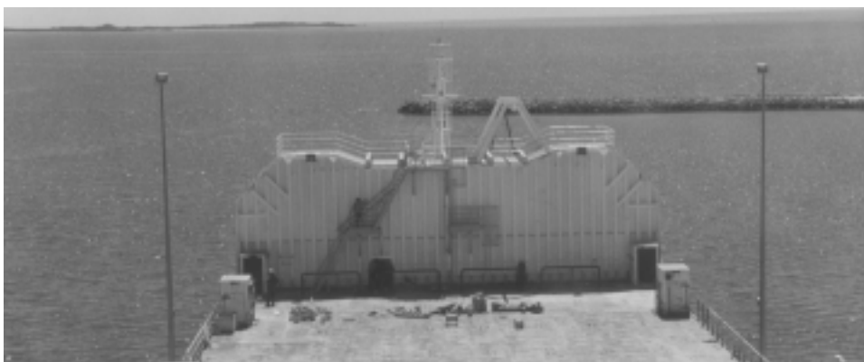
The view forward from the bridge, after fitting the Roll Damping Tank (above)
