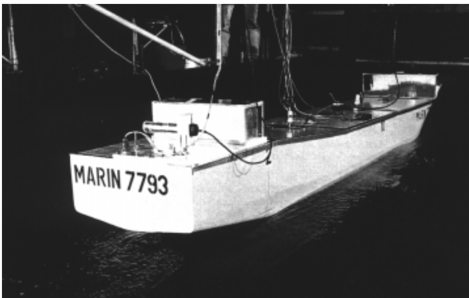
The MARIN model in the same condition, stabilised, in regular beam seas (below)
