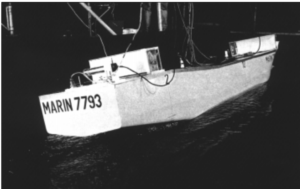
The MARIN model - unstabilised rolling in regular beam seas (above)
