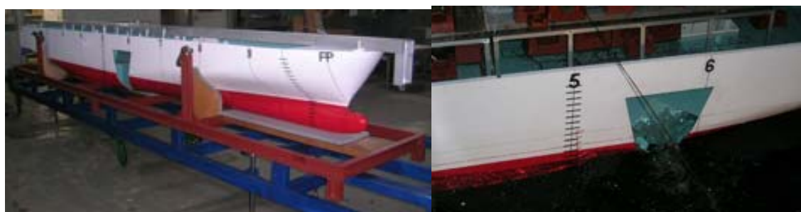
Figure A1 – Photo of model of the RoPax ferry and experiments in beam irregular waves
